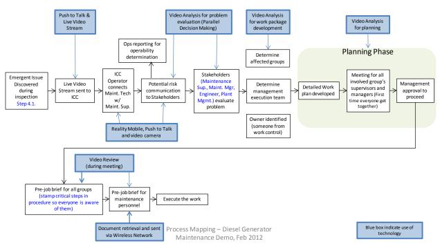
Figure 4. Diesel generator maintenance demonstration process map.
